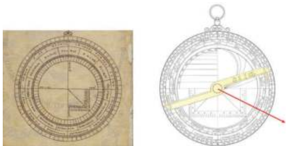
Figure 4 Left: Drawing of the backside of an astrolabe showing a shadow-quadrant in a manuscript dating from before 1054, written by Hermann of Reichenau ( Bibliotheca Vaticana , lat. 598 f. 119'). Right: Accurate sketch of the backside of an astrolabe including the alidade. The red arrow indicates a possible direction of the line of sight [20] representing an angle for which the horizontal length is twice as long as the vertical length.
