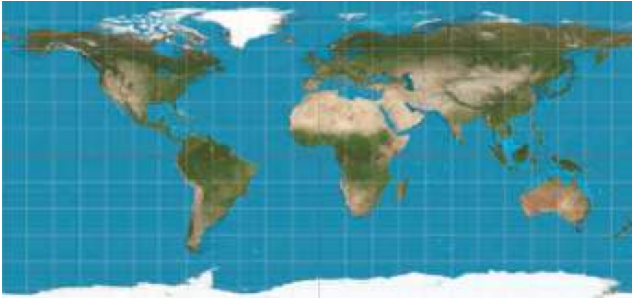
Figure 3 World map on the equidistant cylindrical projection centred on the equator. The graticule interval is 15°.
