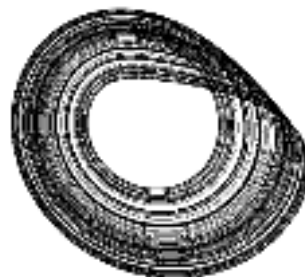
Figure 9 The Rössler attractor projected on a plane.
