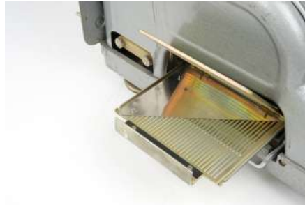
The equivalent of the plugboard on the Fialka. Have you ever seen a physical identity matrix?!
