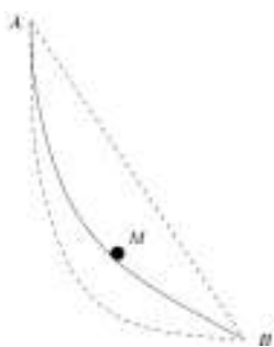
Figure 2 Imagine that you are trying to connect two points A, B in a vertical plane by a slide along which a point mass M will move, solely under the influence of gravitation, in shortest time from A to B .
