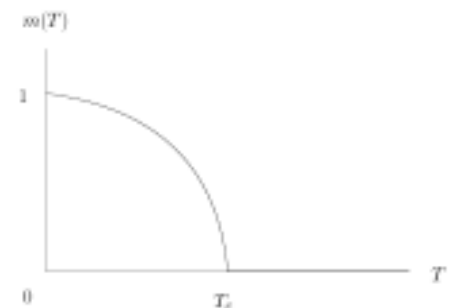
Figure 1 Spontaneous magnetisation: the magnetisation m(T) as a function of the temperature T for a typical configuration of the spins; m(T) is the difference between the number of up-spins and the number of down-spins divided by the total number of spins. The characteristic feature of ferromagnets is that there is a critical temperature , T_c , below which the spins exhibit collective behaviour in that a majority of them point in the same direction (either a majority up or a majority down). By symmetry, configurations with the opposite magnetisation -m(T) are equally likely.
