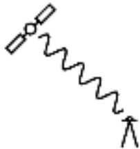
Figure 3 Measurement of phase on the continuous carrier wave transmitted by the satellite. The satellite keeps on transmitting the carrier wave, cycle after identical cycle.
