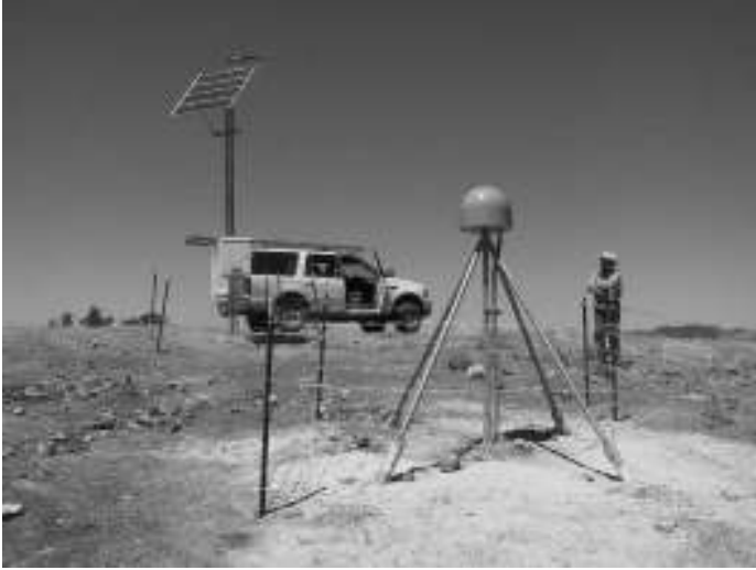
Figure 2 A GPS receiver and antenna permanently installed for precisely monitoring motions of the earth's crust. Site Ranchita in California in the US. Photo taken from album at http://www.scign.org/
